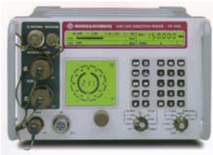
Fig. 13: Doppler direction finder for portable use in frequency range 20 MHz to 1000 MHz
