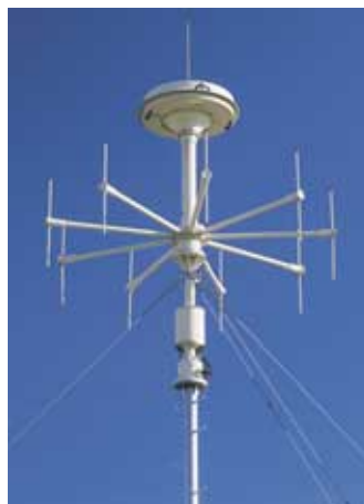
Fig. 16: Direction Finder DDF06M (photo 42136) operating on the principle of a correlative interferometer for the frequency range 20 MHz to 3000 MHz. Nine antenna elements are used for each of the three frequency sub-ranges (photo 43073-2)
